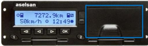
Inside the printer drawer there is a printer mechanism that holds printer and a roll of paper. The printed paper will come out from a small opening at the top of the printer drawer.
