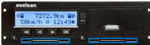
The card slot for the driver is on the left and card slot for the co-driver is on the right. Each card must be inserted all the way to the stop. The cards are locked mechanically and normally they can only be removed electrically with the help of the user action (long pressing the **keypad #1** and **keypad #2** ) when the vehicle is stationary.
