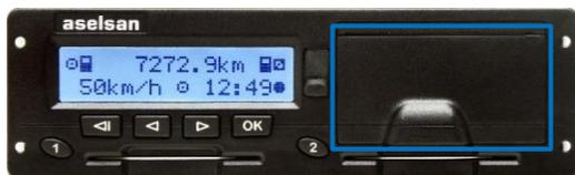
Inside the printer drawer there is a printer mechanism that holds printer and a roll of paper. The printed paper will come out from a small opening at the top of the printer drawer.
